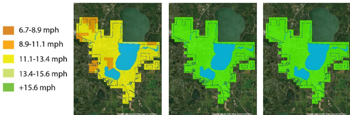
Figure 10 Wind speeds at different tower heights, 30 meters, 80 meters, and 100 meters from left to right.
